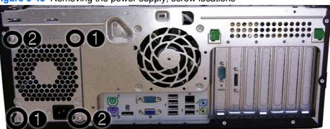
Figure 5-43 Removing the power supply, screw locations
